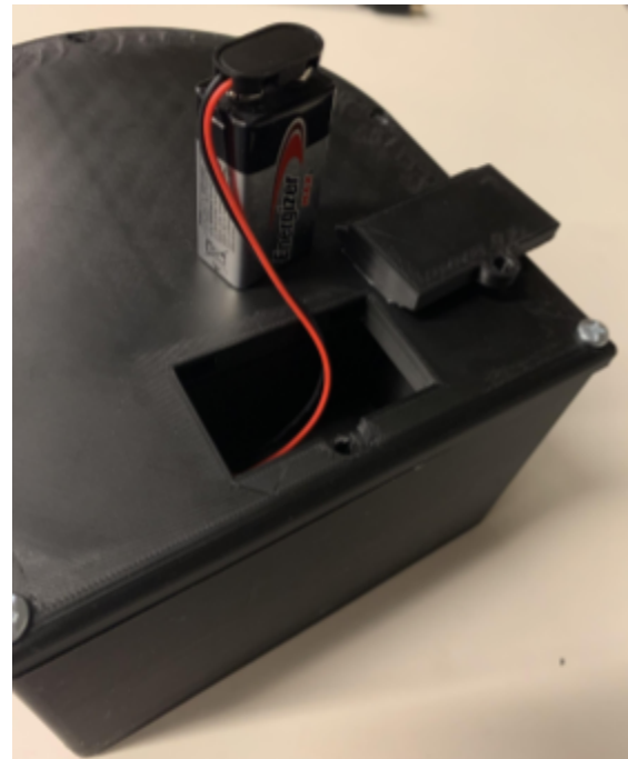
Figure 14: Battery for Target
